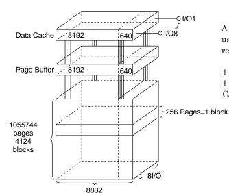
A page consists of 8832 bytes in which 8192 bytes are used for main memory storage and 640 bytes are for redundancy or for other uses.
